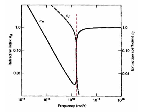
Figure 27-3 Angular frequency dependence of the refractive index  $n_R$  and the extinction coefficient  $n_I$  for copper. Values assumed are  $\omega_p = 1.63 \times 10^{16} \text{ s}^{-1}$  and  $\gamma = 4.1 \times 10^{13} \text{ s}^{-1}$ . The crossover point of the curves coincides with the plasma frequency.
